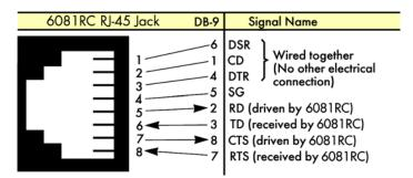
Figure 10. DB-9-to-RJ-45 cable diagram
